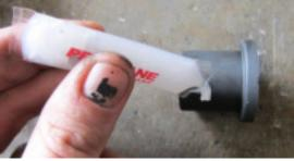
6) With both urethane ends now in place you will slide in the center sleeve. Coat the sleeve with
