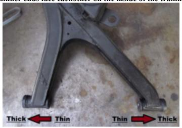
5) Spread a liberal amount of the supplied lube (it is a non-corrosive silicone-based di-electric grease) on one half of the bushing and sliding it into the trailing arm. Repeat with the other end. Do NOT install the center sleeve prior to having both urethane ends in place.
