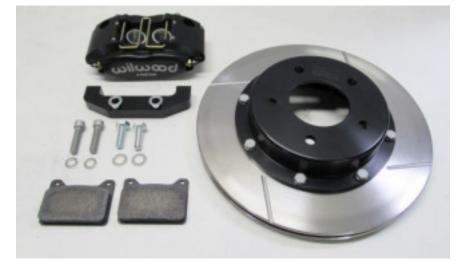
3) Rotor orientation. The slots (and interior venting) are angled so that during forward movement hot gases will be pushed out and away from the rotor a la centrifugal force (imagine that roundabout you rode on at the playground as a kid).
