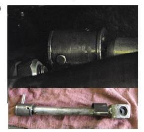
8) At the forward end of the shift linkage is the selector rod coupler. There is a cylindrical metal spring which covers the outside of the coupler. You will need to pry away and remove this spring to access the dowel which connects the coupler to the transmission. The dowel slides vertically out of the coupler, and can be pushed out using a suitable drift. See pictures on right.
