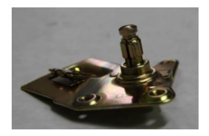
As shown in the picture install the bolt with the handle off and make it just snug, but not too tight which would spread the prongs too wide for the handle to be put on. This will keep the prongs sturdy enough to handle the pressure from the set screw(s) and keep your handle or crank on. Then just place the handle/crank over the bolt and splines and set the screw(s).
